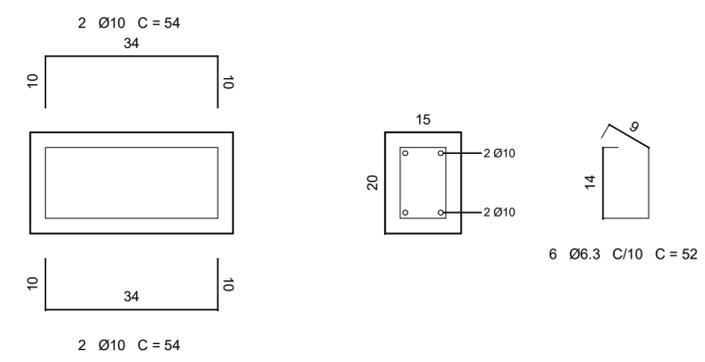
**DETALHE ARMADURA COXIM DE CONCRETO**
