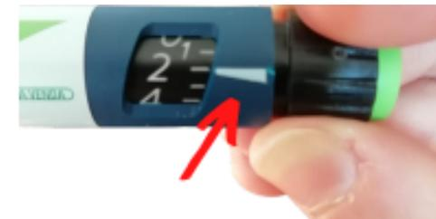
APONTANDO A CANETA COM A AGULHA VIRADA PARA CIMA, PRESSIONE O BOTÃO INJETOR. UMA GOTA DEVE APARECER NA PONTA DA AGULHA E O SELETOR DE DOSE DEVE RETORNAR AO "0" (ZERO)
